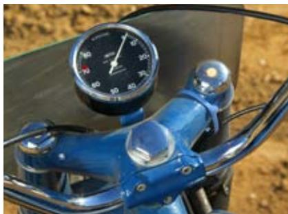
An unusual, upside-down Smiths tachometer features a needle that sweeps around the bottom of the gauge. Redline is 7000 rpm, where the 500cc single makes 52 bhp.
