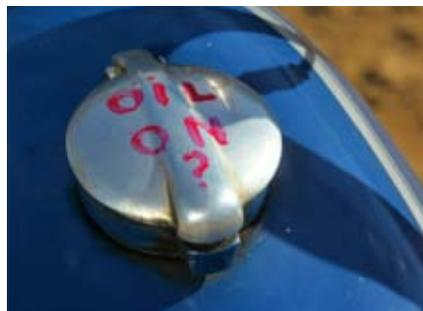
In addition to the fuel petcock, the feed line from the remote oil tank also has to be turned on before starting the bike. Forgetting to do so can be a costly mistake.
