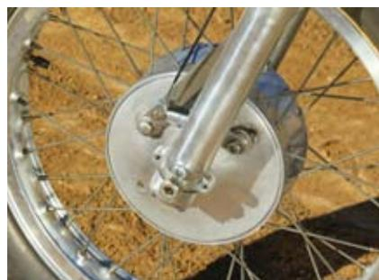
The bike is fit with a single-shoe drum front brake, but Rayborn reportedly rarely used it. He much preferred to scrub off speed by plowing the front wheel.
